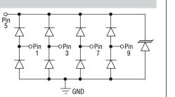
CDDFN10-3304NA - TVS/Steering Diode Array
