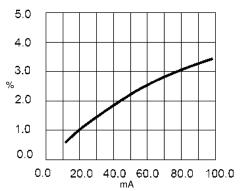
Relative Luminous Intensity vs. Forward Current
