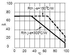
Maximum Forward DC Current vs. Ambient **Temperature**
