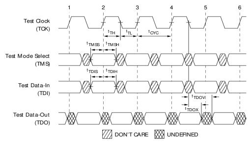
TAP AC Switching Characteristics Over the operating Range<sup>[9, 10]</sup>
