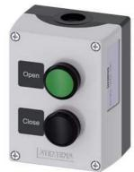
enclosure for command devices, 22 mm, round, enclosure material plastic, enclosure top part gray, 2 control points plastic, B=Pushbutton green, label: Open, 1 NO, screw terminal, A=Pushbutton black, label: Close, 1 NO, screw terminal, floor mounting, 1xM20 each on top and bottom, Labels glued in
