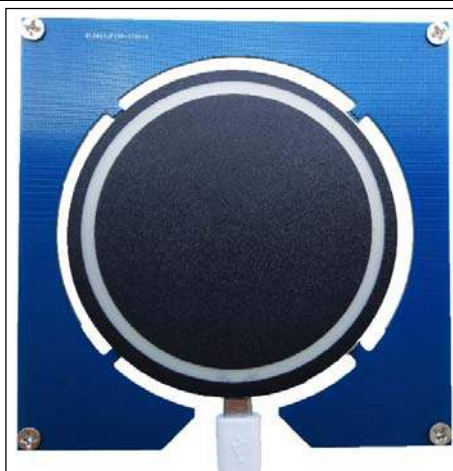
Figure 1: Photo of IS31FL3236A Evaluation Board
