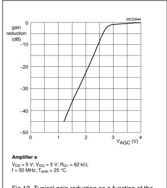
Fig.12 Typical gain reduction as a function of the AGC voltage; see Fig.35.
