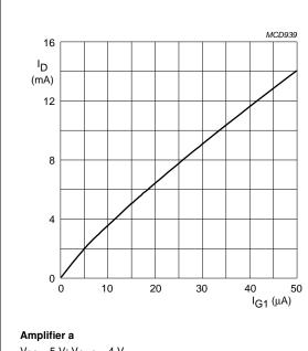
$V_{DS} = 5 \text{ V}; V_{G2-S} = 4 \text{ V}.$  $T_j = 25 \, ^{\circ}\text{C}.$
