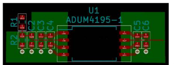
Figure 30. Placement of Decoupling Capacitors, Ground Plane GND 1 , and Ground Plane GND 2
