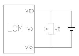
V<sub>DD-</sub>V<sub>0</sub>: LCD Driving voltage VR: 10k~20k
