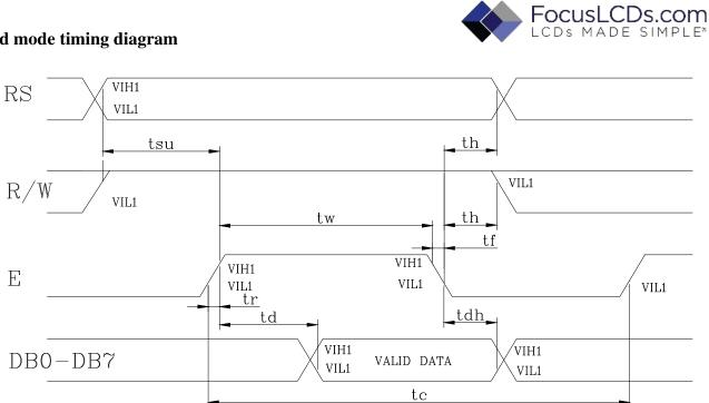
Write cycle (Ta=25°C, V<sub>DD</sub>=5.0V)
