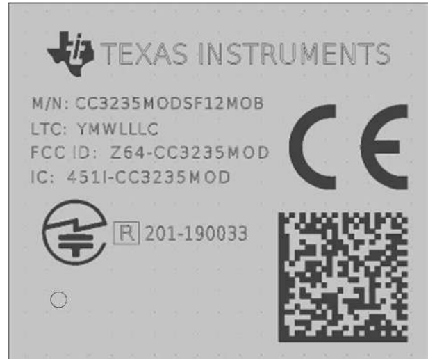
Figure 9-4. CC3235MODSF Module Marking
