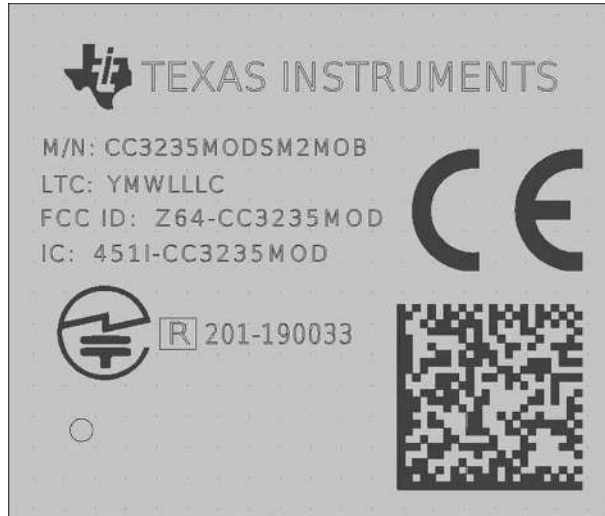
Figure 9-3. CC3235MODS Module Marking
