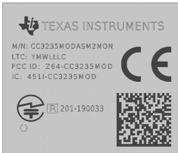
Figure 9-5. CC3235MODAS Module Marking
