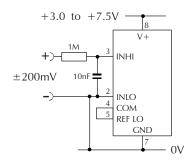
Measuring a single ended input voltage referenced to supply, i.e. the input voltage and the meter's power supply share the same 0V rail. Ensure solder link LREF is closed.
