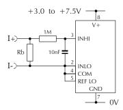
Measuring a current from a circuit which is floating with respect to the DPM's supply, i.e. the current and the meter's power supply are isolated from each other.
