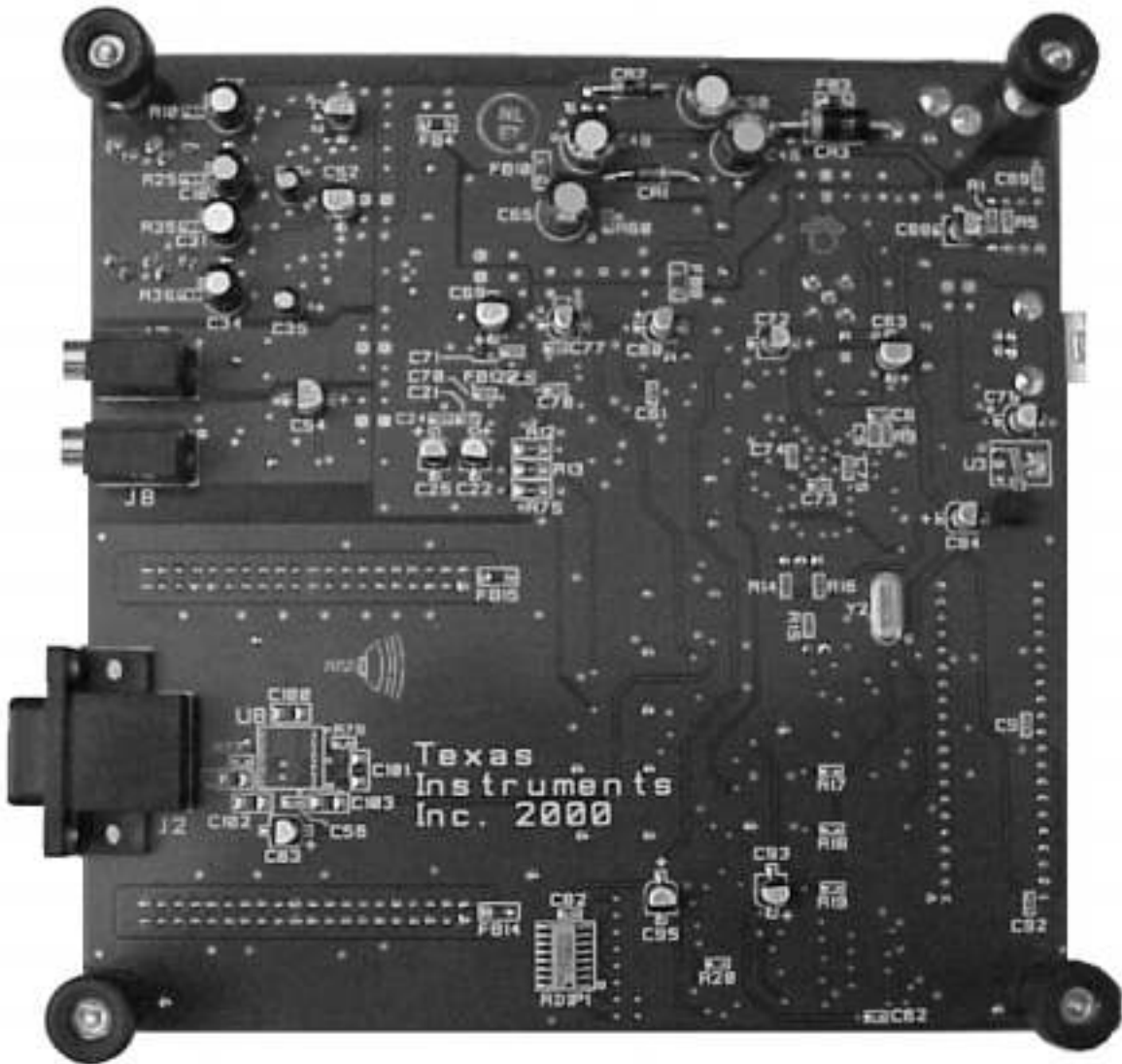
Figure 2–2. TAS1020A EVM Bottom View
