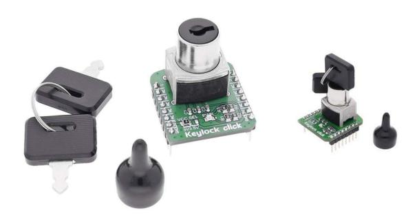
**Keylock click** carries a processed sealed key lock mechanism that can be set in three different ositions. The click is designed to run on either 3.3V or 5V power supply. It communicates with the target microcontroller over the PWM, INT, and AN pin on the mikroBUS<sup>TM</sup> line.
