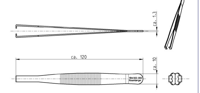
All dimensions are in mm; tolerances according to ISO 2768 m-H
