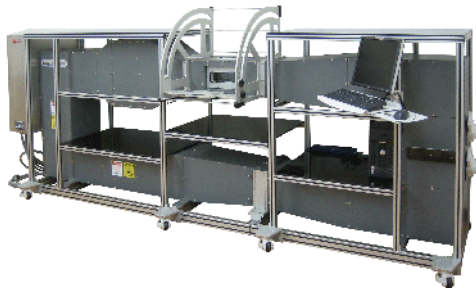
Fig F: FDK Original Wind Tunnel
