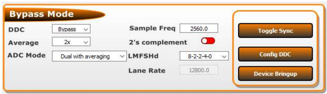
Figure 3-2. Bypass Mode Settings
