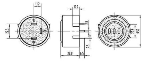
Only when apply  $12V_{DC}$  on pin "c", the product can produce sound
