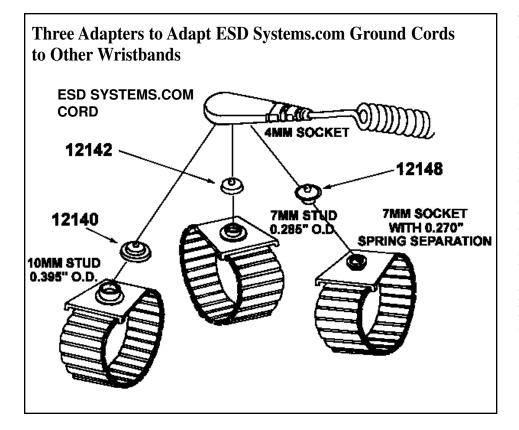
There are three connector systems commonly used for ESD protective grounding. These are the 4mm (1/8"), 7mm (1/4") and 10mm (3/8") snap. These are available in both male (stud) and female (socket) snaps.
