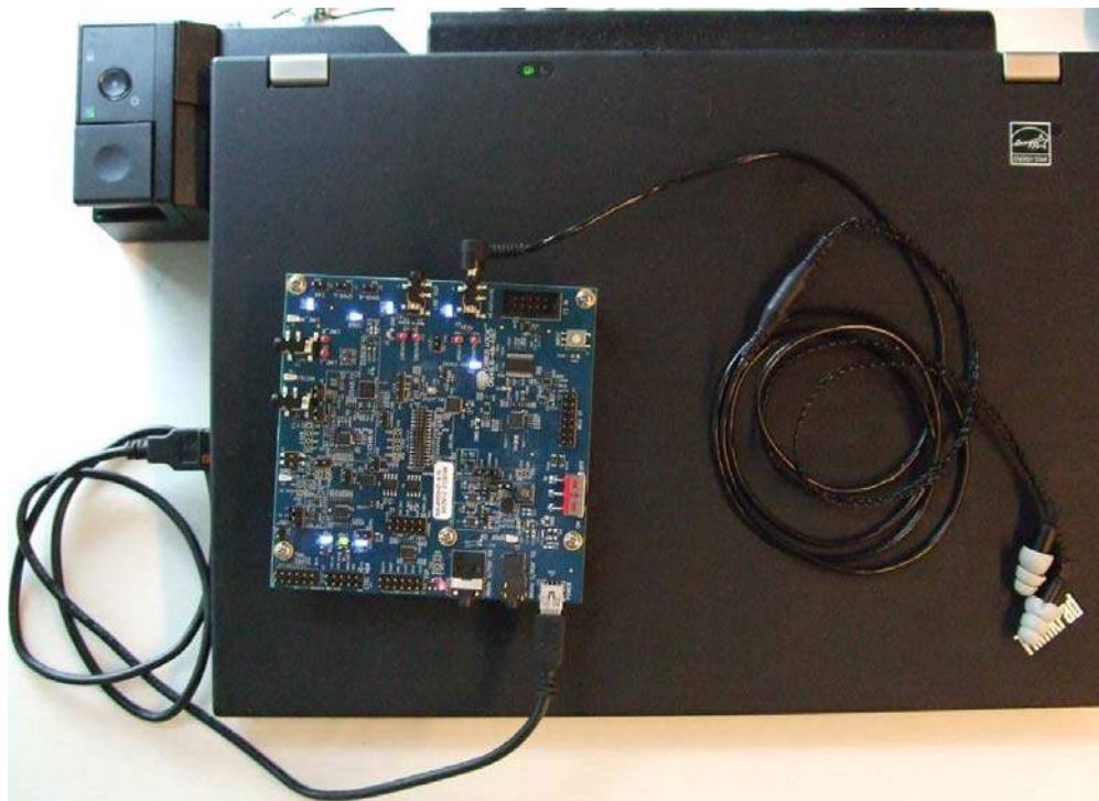
Figure 4-1. CRD48L10-4in4out Powered by PC, Configured for MP3 Playback over SPI
