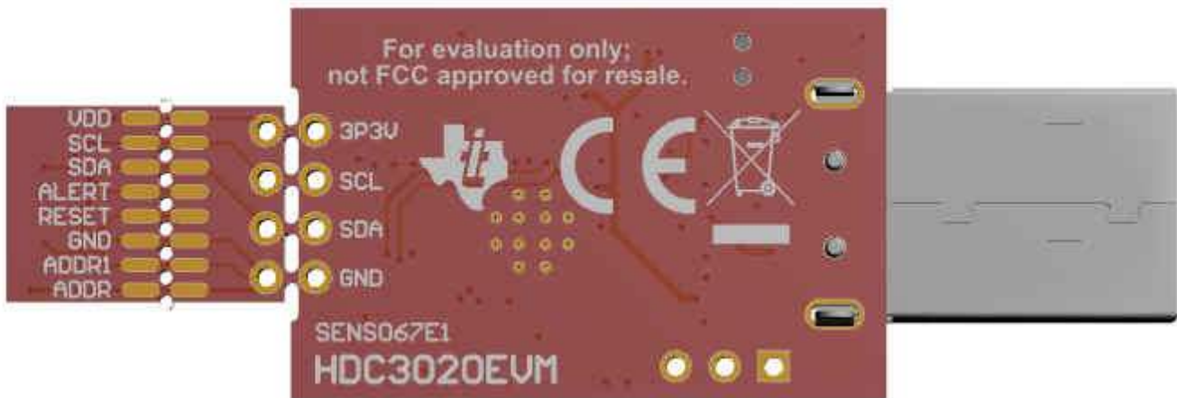
Figure 3-5. Bottom Layer of the HDC3020EVM
