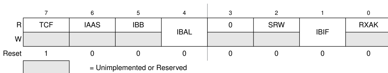
Figure 12-7. IIC Bus Status Register (IBSR)
