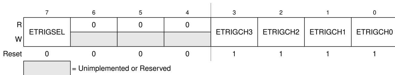
Figure 7-4. ATD Control Register 1 (ATDCTL1)
