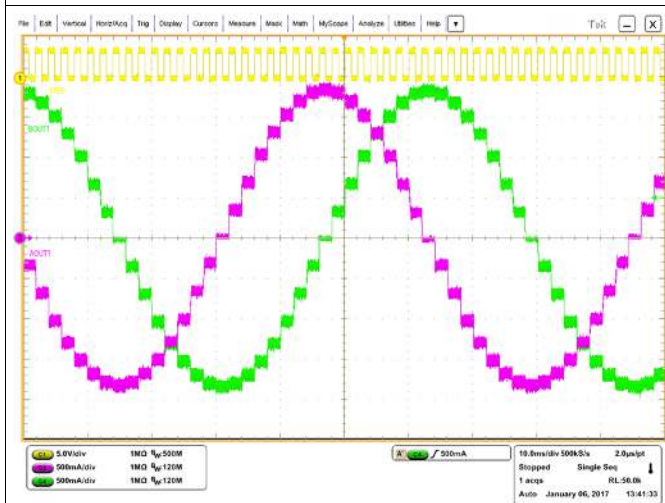
Figure 27. 1/8 Microstepping With Slow-Slow Decay; Loss of Current Regulation on Falling Steps
