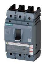
circuit breaker 3VA5 UL frame 250 breaking capacity class M 35kA @ 480 V 3-pole, line protection TM230, FTAM, In=110A overload protection Ir=110A fixed short-circuit protection Ii=5...10 x In UL 489 SB (naval), 50° C without connection
