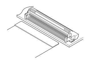
The connector for the 0.3 mm thickness FFC or FPC with a mounting height of 2.0 mm. This 0.5 mm pitch FFC or FPC connector adopts a ZIF structure, which provides superior performance in durability and offers effective protection from wearing. The use of the rotating type cover contributes to easy operation especially with big circuits connectors.
