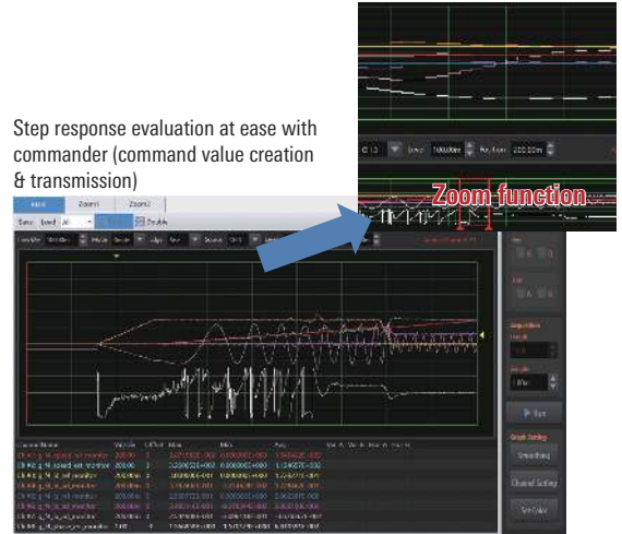
Display variables for 8 channels (can specify scale and off-set settings etc. per channel)
