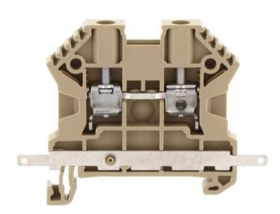
Feed-through terminal, Screw connection, Mounting type: Mounting rail TS 35/7.5, Rated cross-section: 4 mm², Width: 6 mm, Colour: White
