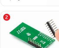
Turn the board upside down so that bottom side is facing you upwards. Place shorter parts of the header pins in both soldering pad locations.
