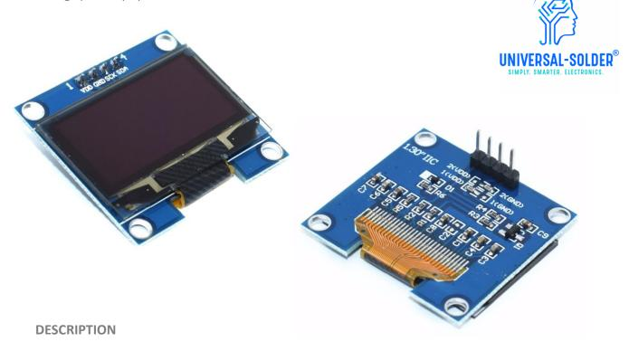
These displays come with SSD1306 or SH1106 controller, but the actual model is not disclosed. Libraries are available for both controllers, and we recommend a library that works for both controller types.
