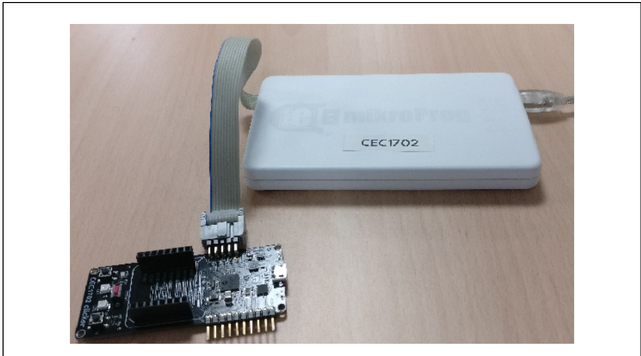
FIGURE B-1: CEC1702 CLICKER BOARD SETUP
