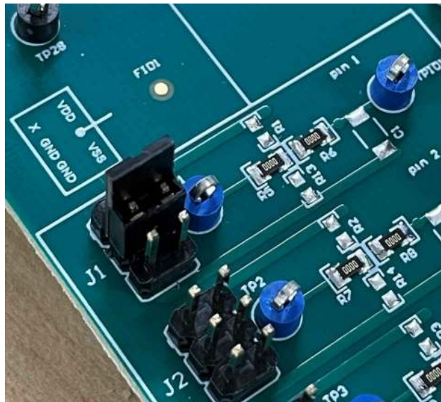
Figure 6-2. Signal Line Circuitry (3D)
