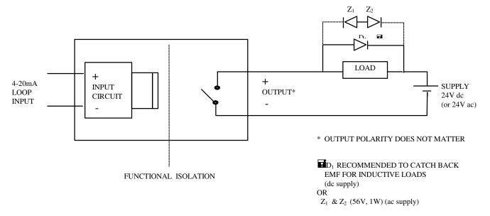
**BLOCK DIAGRAM: 24V ac/dc RELAY VERSION**
