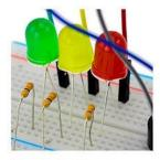
Simple Build No soldering here! Simply slot the components into the breadboard... and pull them right out again.
