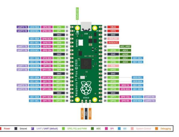
The Raspberry Pi Pico board, a new low cost, high-performance microcontroller. The board features a powerful new, Raspberry Pi designed ARM-based dual-core chip-- the RP2040. The pico also features 64KB of internal RAM and support for up to 16MB of off-chip Flash. A wide range of flexible I/O options includes I2C, SPI, and Programmable I/O (PIO). These support endless possible applications for this small and affordable board.
