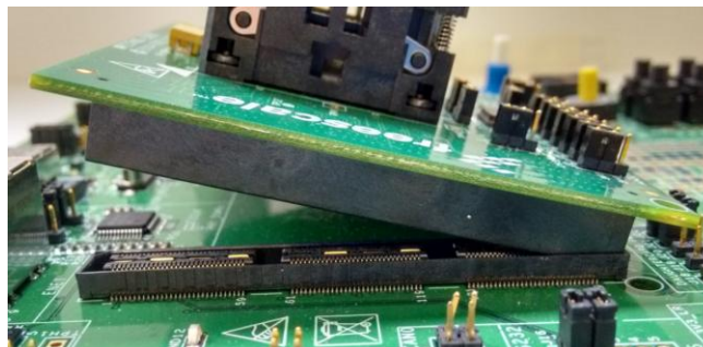
Figure 3. Removing a daughtercard
