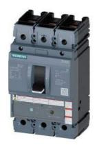
circuit breaker 3VA5 UL frame 250 breaking capacity class C 100kA @ 480 V 3-pole, line protection TM240, ATAM, In=100A overload protection Ir=80A ...100A short-circuit protection Ii=5...10 x In nut keeper kit on both sides
