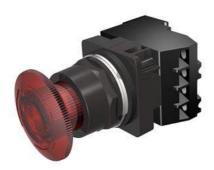
30mm BlackMax, Epoxy Coated Corrosion Resistant Complete Metal Unit Illuminated Twist-to-Release Full Voltage, 24V AC/DC Incandescent Lamp Mushroom Head Cap Small 1.79" (45 mm) Plastic Cap, Red 2 Position Maintained, Twist-to-Release with 1 N.O. - 1 N.C. Heavy Duty Contacts, A600/P600 UL Listed, CSA Certified NEMA 1,3,3R,4,4X,12,13 & Automotive Standards
