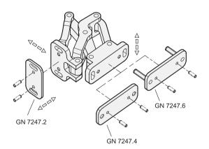
Multiple-joint hinges can be adjusted in three planes during installation. For example, this allows compensation for tolerances or establishing of required compressive forces for seals.
