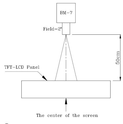
2 The Brightness Test Point Setup
