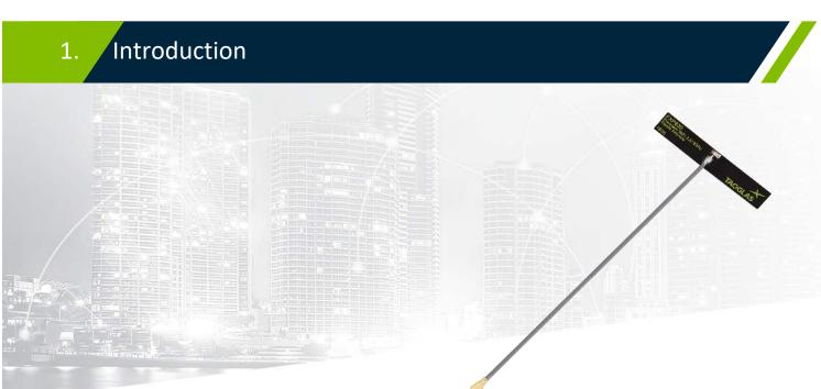
The FXP830 is a high efficiency, small, dipole antenna covering 2.4/5.8/7.1GHz bands including Bluetooth, Wi-Fi and the newly established Wi-Fi 6/Wi-Fi 6E, making this an ideal solution for future-proofing an IoT device. This Taoglas patent pending antenna is unique in the market because it is made from poly-flexible material, has a tiny form factor (42\*7\*.01mm) and has double-sided 3M tape for easy "peel and stick" mounting.
