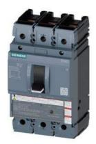
circuit breaker 3VA5 UL frame 250 breaking capacity class M 35kA @ 480 V 3-pole, line protection TM230, FTAM, In=100A overload protection Ir=100A fixed short-circuit protection Ii=5...10 x In UL489 SB (naval), 50 deg. cel. nut keeper kit on both sides
