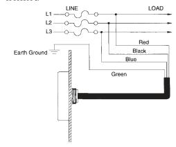
The ATC Diversified Electronics **GFD Series** is intended for the use on ungrounded systems to detect and indicate the phase of the first ground fault condition. This enables corrective action to avoid the potential hazards resulting from a second ground fault.
