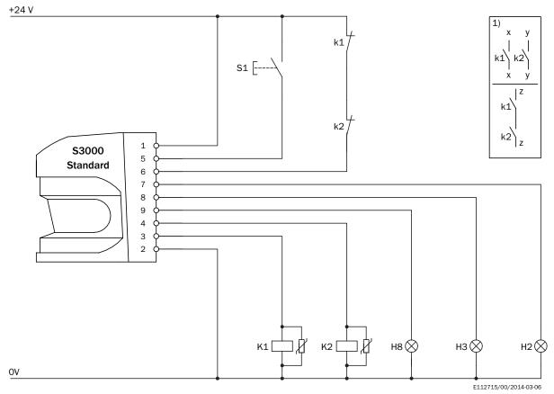
S3000 Standard in conjunction with relays/contactors
