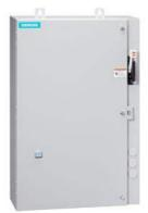
Non-reversing motor starter Size 0 Three phase full voltage Solid-state overload relay OLRelay amp range 0.25-1A 24VAC 50-60HZ coil Combination type 30Amp fusible disconnect 30 Amp /600V fuse clip Enclosure NEMA type 4/12 Water/dust tight weather proof Extra-wide enclosure
