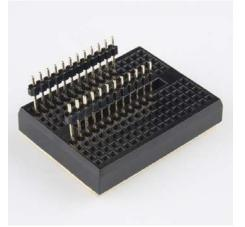
Once the pin headers are in place, you can lower the MiniGen board onto them. The board can be soldered on component side up or component side down; depending on what you plan to do with it, one of those is likely to be better.
