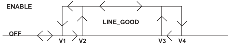
Figure 2. Line UVLO and OVLO Operation
