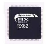
The **uEZGUI-RX62N-35QT** includes a 96MHz Renesas RX621 or RX62N microcontroller running the open source uEZ® + FreeRTOS software platform. The RX62N has 512KB of internal Flash memory, 96KB of internal SRAM, a 10/100 Ethernet Media Access Controller (MAC), a USB full speed device/host/OTG controller, up to six UARTs, one CAN channels and a collection of serial communications interfaces.
