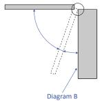
The damper torque becomes larger, preventing the lid from closing completely
