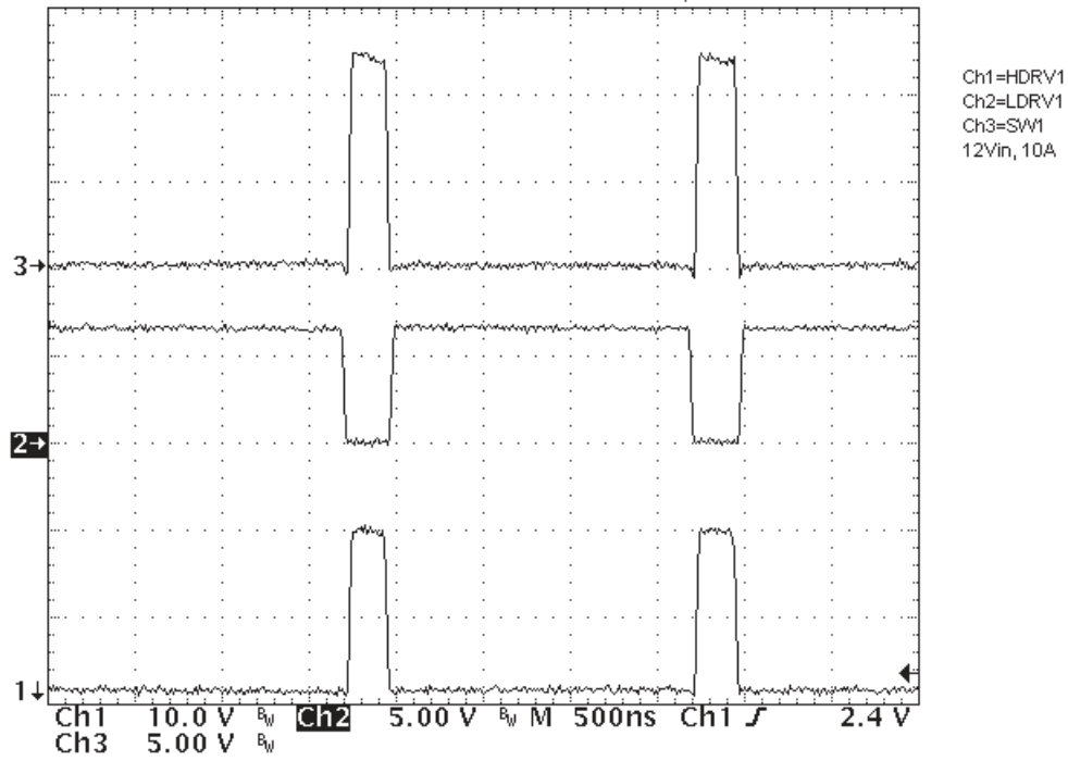
Figure 14. Output 1 Switching waveform, (Ch1 = HDRV1, Ch2 = LDRV1, Ch3 = SW1, VIN = 12 V, I OUT1 = 10 A)
