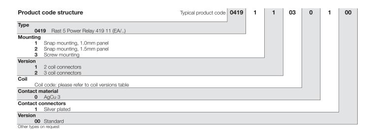
**Product code** Cont. material Version Cont.arrangement Coil Part number 0419 11 0301 00 Snap Mounting AgCu3 2 form A, 3-1415419-5 AC coil 2 NO 4-1415419-0 0419 11 1201 00 1.0mm plate DC coil 0419 11 1301 00 contacts 4-1415419-2
