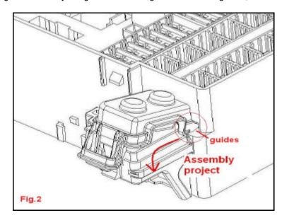
c) Close the Cover Eyelet pushing in the direction shown on Figure 3 to final position (CLICK).
