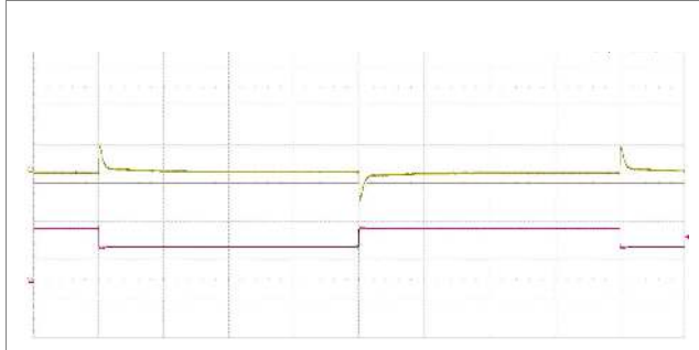
Output voltage response to load current step- change (1.0-1.5-1.0 A) at: T_{P1} = +25^{\circ}\text{C} , V_i = 110\text{ V} . Top trace: output voltage (500 mV/div.). Bottom trace: load current (1 A/div.). Time scale: (2 ms/div.).
