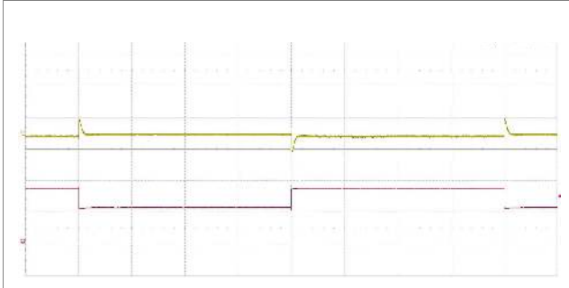
Output voltage response to load current step-change (1.25-1.875-1.25 A) at: T_{P1} = +25^{\circ}\text{C} , V_i = 110\text{ V} . Top trace: output voltage (200 mV/div.). Bottom trace: load current (1 A/div.). Time scale: (2 ms/div.).
