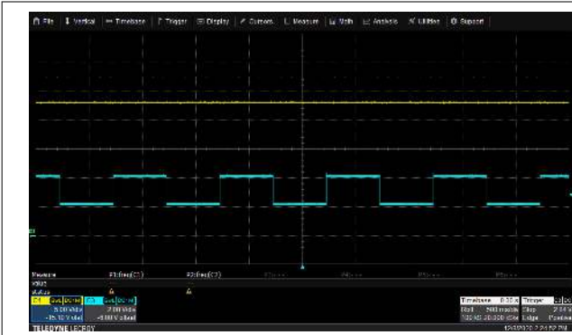
Figure 6-13. Load Transient Response, measured between TP6 and TP7 (a. no V_{OUT} deviation observed due to the LDO; b. V_{OUT} = 23V )
