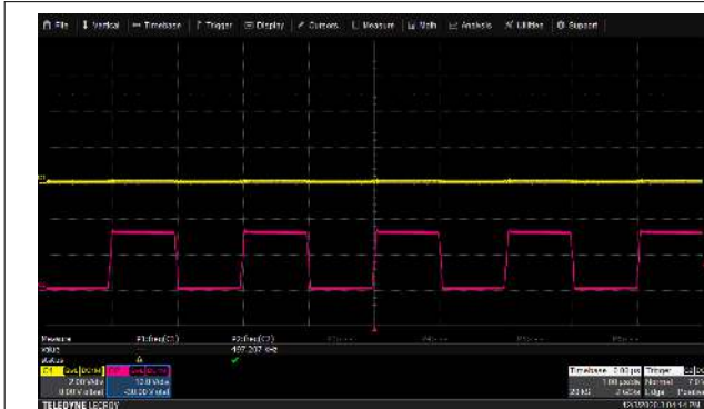
Figure 6-9. Fsw = 497 kHz without external sync
